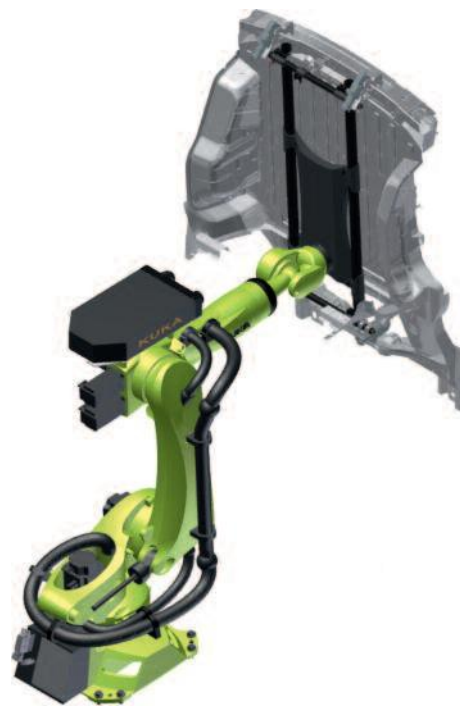
Example application – transporting 115 kg floor pan
