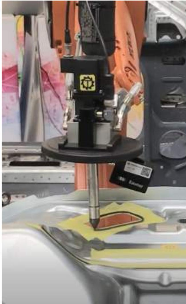
*More than 80 % of all standard dosing applications are done with relatively simple seams applied on a part. Furthermore, most of the times the width of the seam is not changed during an applicated seam. Exactly for those applications we developed a stable process, where the adhesive or sealer is pumped directly from the TÜNKERS electrical pump station trough the robot mounted TÜNKERS electrical application head and finally on the part. Totally without the usage of any doser.*
