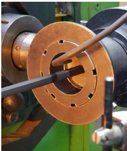
Extrusion die: Extruder with emerging elastomer profile
