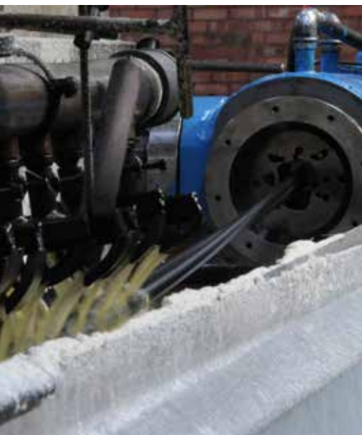
220° salt bath to accelerate the vulcanization process
