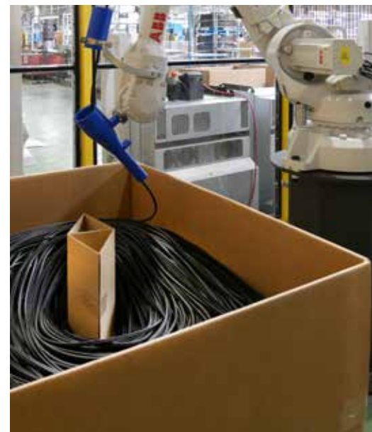
Robot-controlled insertion of the profile into bulk packaging
