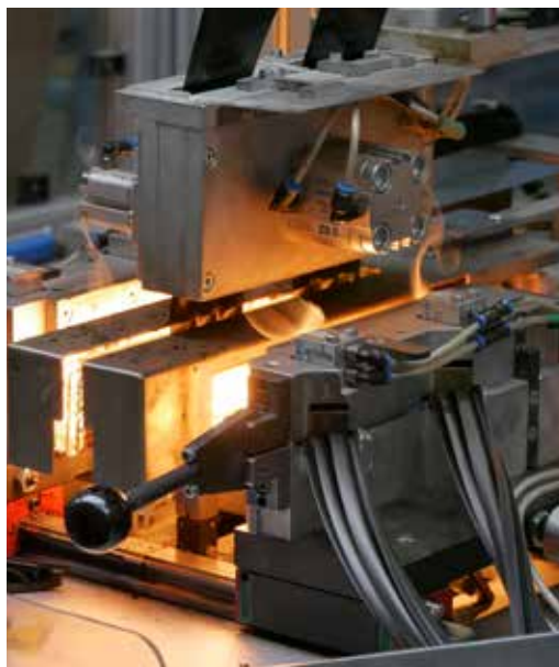
PE film welding for rings and frames
