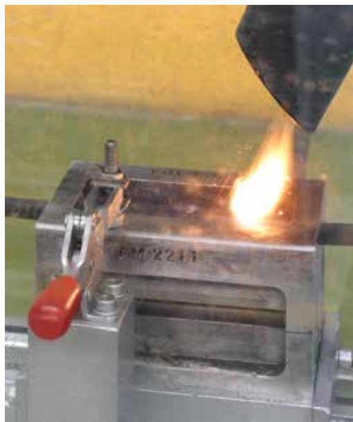
Laser marking of the elastomer profile according to customer requirements
