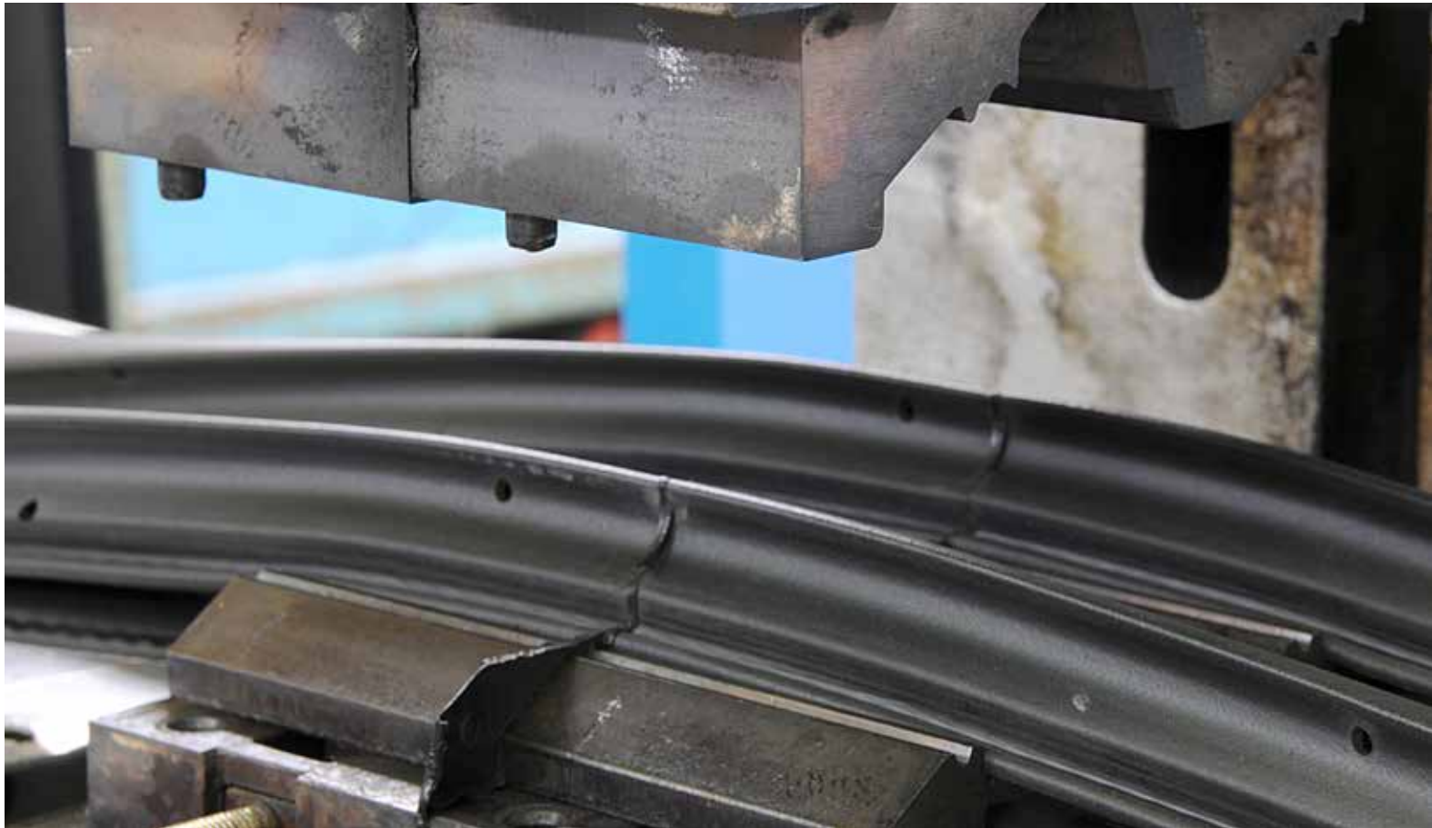
EPDM film vulcanization for rings and frames
