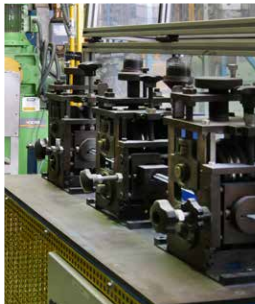
Bending roller set for profiling the metal insert
