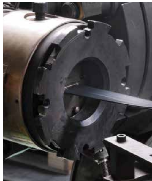
Extrusion die: Extrusion with emerging PVC profile
