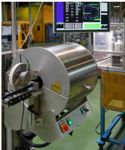
Permanent camera-based profile geometry monitoring (PIX-Argus)
