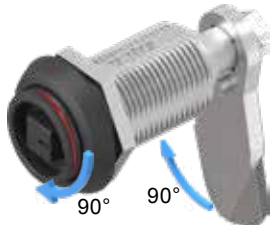
Open condition Turning the insert 90° causes the cam to rotate.
