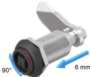
Closed condition Further rotation of the insert by 90° moves the cam 6 mm in axial direction.
